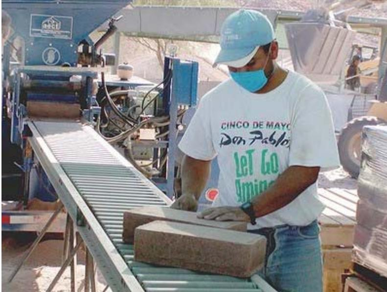
The earthen mixture is compressed into building blocks
