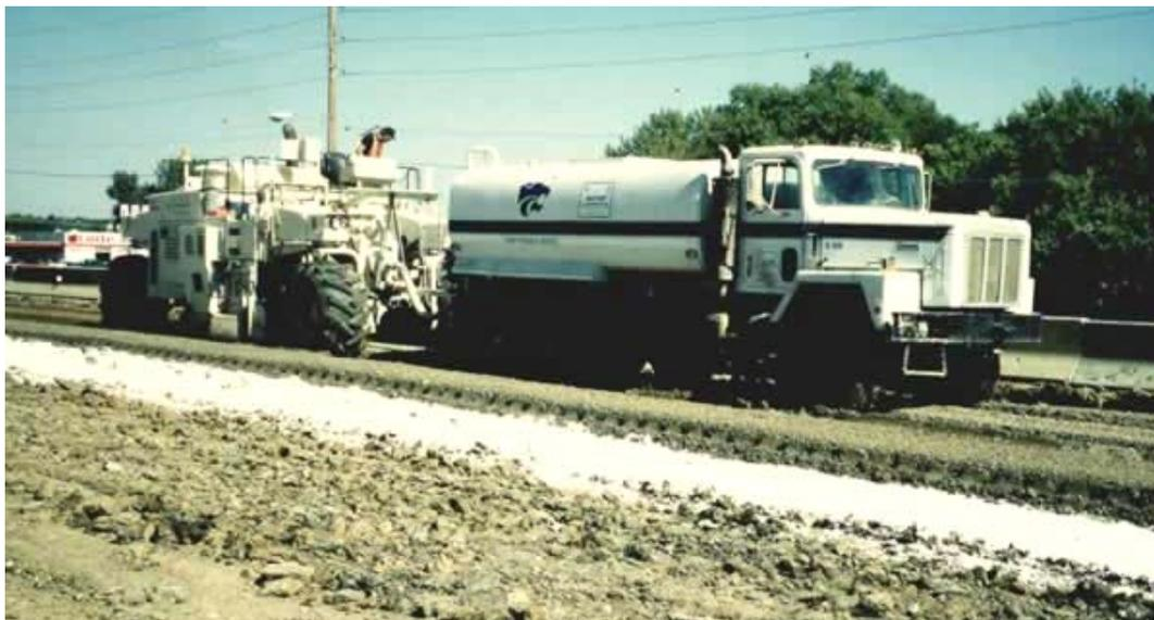
Figure 15: Rotary mixer with water truck attached
