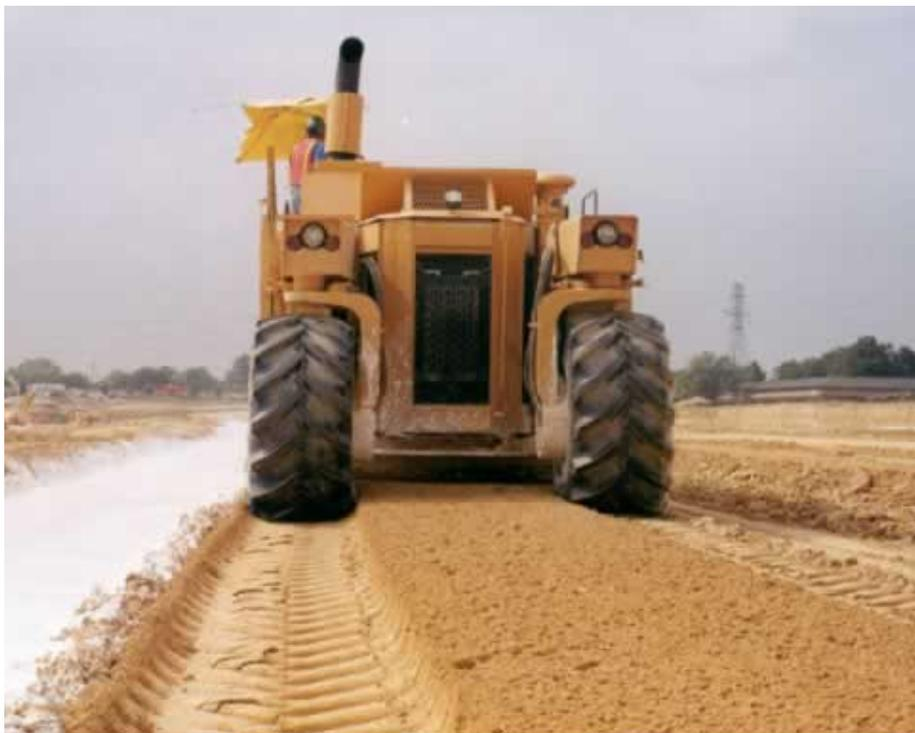
Figure 14: Rotary mixer used for initial mixing
