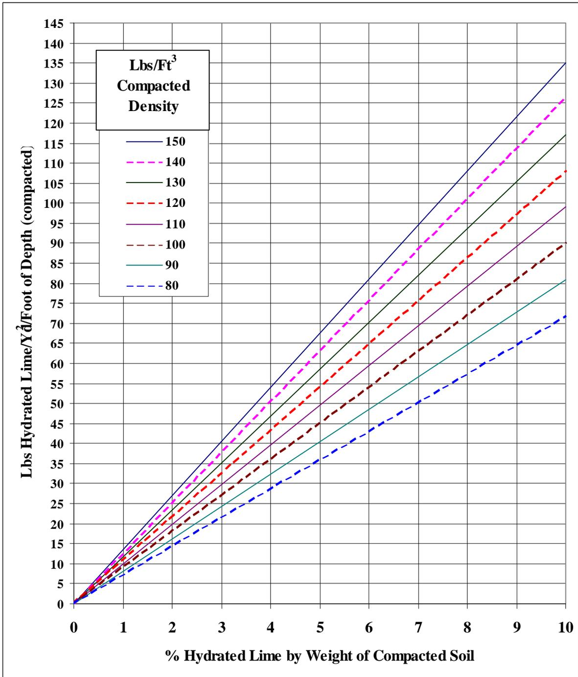
Figure 25: Graphical Conversion for Hydrated Lime Application Rates
