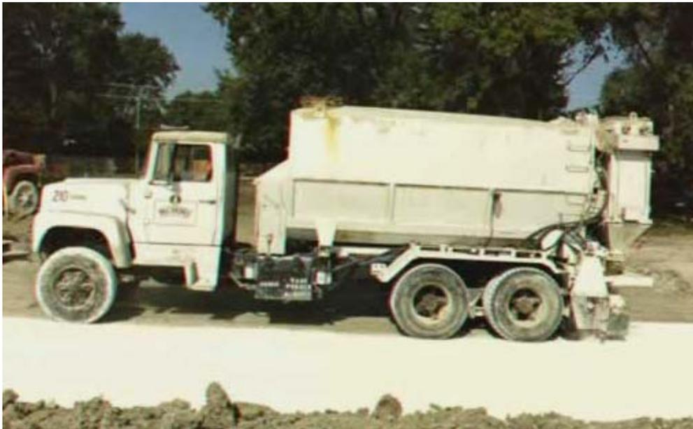
Figure 10: Dry lime application with mechanical spreader<sup>4</sup>
