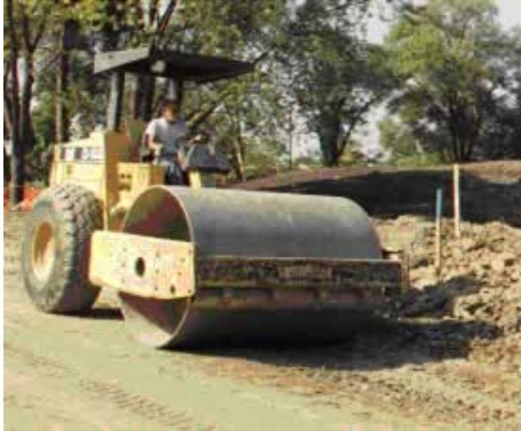
Figure 18: Steel roller
