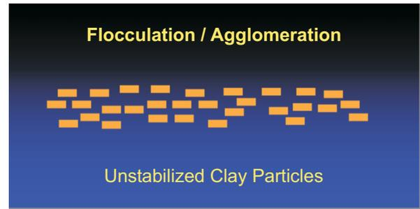
Untreated clays have a molecular structure similar to some polymers, and give plastic properties. The structure can trap water between its molecular layers, causing volume and density changes.
