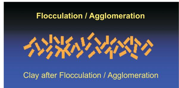
In treated clays, calcium atoms (from lime) replace sodium and hydrogen atoms producing a soil with very friable characteristics.
