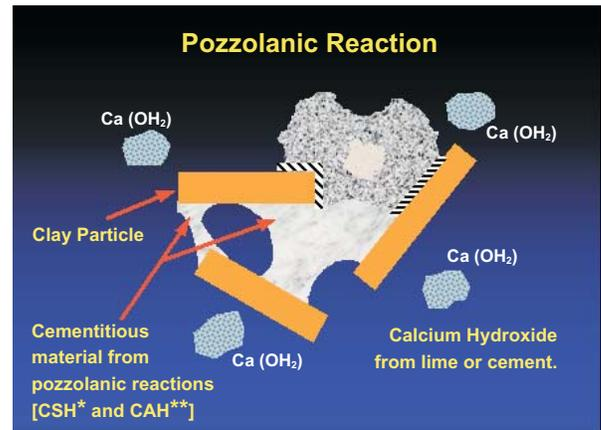
On-going reaction with available silica and alumina in the soil forms complex cementitious materials--the POZZOLANIC effect.
