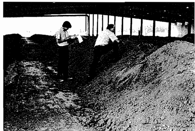
Fig. 2 — Windrow composting of lime-treated sewage sludge at Upper Occoquan Sewage Authority plant.
