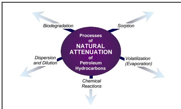
Figure 1. Processes of natural attenuation of petroleum hydrocarbons.
