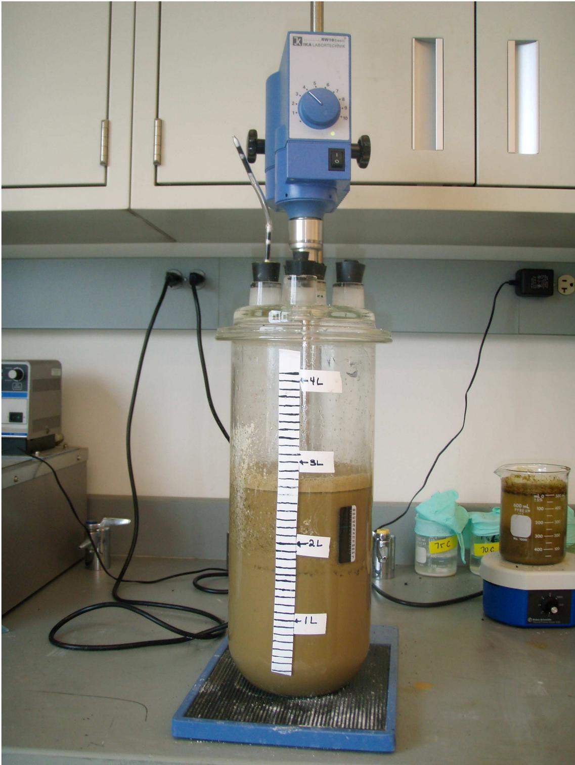
**Figure 1. Picture of the closed slurry reactor set-up, showing the mechanical mixer, the lid with ports, and the two activated carbon traps in series.**
